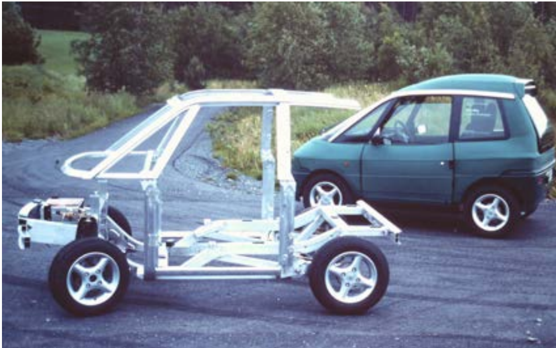
The aluminium frame of an early PIV3 (the car shown on the next page) together with one of the Winter Olympics cars at Aurskog in April 1994. Only a few of the first cars remained in Norway. (Photo: Håkon Aurlien)
