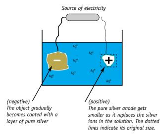
If a silver/copper alloy layer is required, then the appropriate combination of silver and copper salts is dissolved, and the corresponding alloy is used as the anode.
